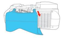
Insert the wireless LAN module into the port.
